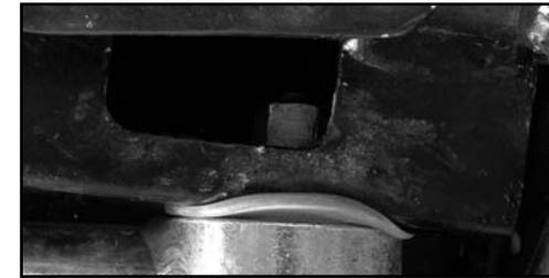
FIGURE 12.1 TRACK BAR BRACKET BOTTOM VIEW, NUT MUST BE INSERTED THRU THE SLOT
