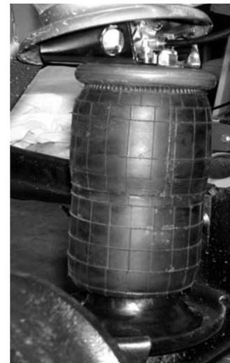
The rear Airspring assemblies are designed to bolt in the stock location as well, as shown. The upper bump stop hole must be drilled to 3/8”, the lower spring plate must have a 1/2” hole put in the center. Remove the rubber upper and plastic lower OEM spring cushions. Insert the airline, again ensuring the proper trim technique is utilized.
