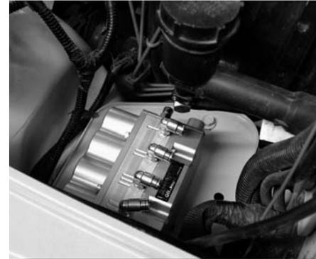
The AiROCK Control Unit (ACU) can be mounted anywhere under the hood, limited only by the wire harness which is designed to have the main junction at the center of the firewall. This unit will have all four airspring airlines run to it as well as the pressure supply line. This unit is shown mounted on the ABS tray, but may be placed almost anywhere in any position.
