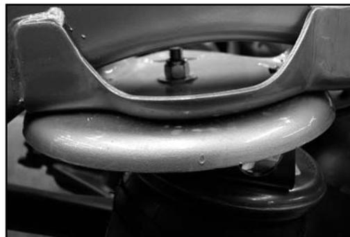
Figure 14.3 Install washer and nut on top mount
