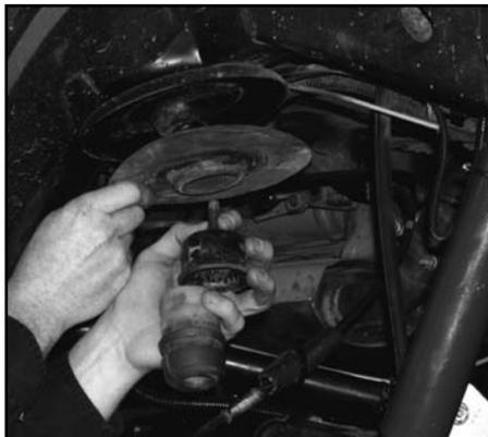
Figure 13.2 Removal of upper hardware
