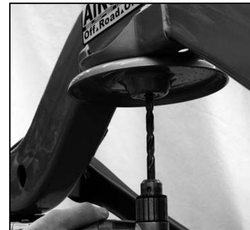
Figure 13.4 Drill upper bumpstop mount threads to 3/8"
