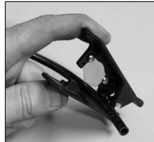
FIGURE 7.2 AIRLINE BEING TRIMMED WITH SUPPLIED TUBING CUTTER
