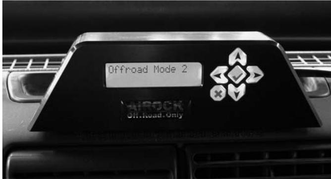
The Controller is designed to be attached to the top center of the dash bezel with the already attached self-adhesive tape. Please clean dash mount thoroughly and prep surface for installation with an alcohol pad. The control cable should be run through the dash and exit on top under the defroster cover.
