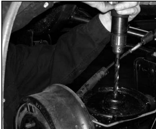
Figure 14.2 Drilling 1/2” Hole in Center of Spring Pad
