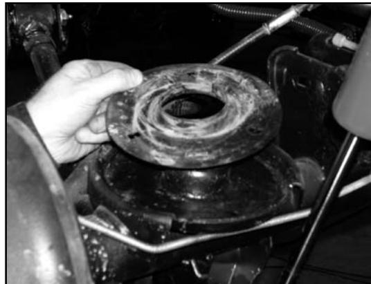
Figure 13.3: Removal of Lower Mount Insert
