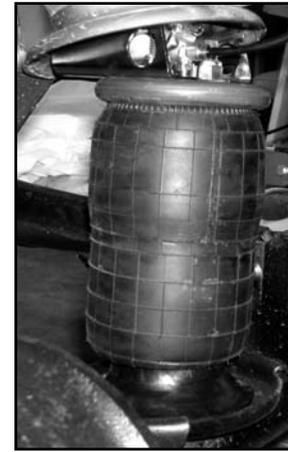
Figure 13.1 Rear airspring installed
