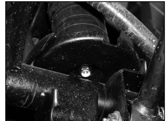
Figure 14.4 Install nut on lower stud
